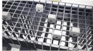
Warehouse Automation Solution i-Hub: Automated Bin Storage Retrieval System
